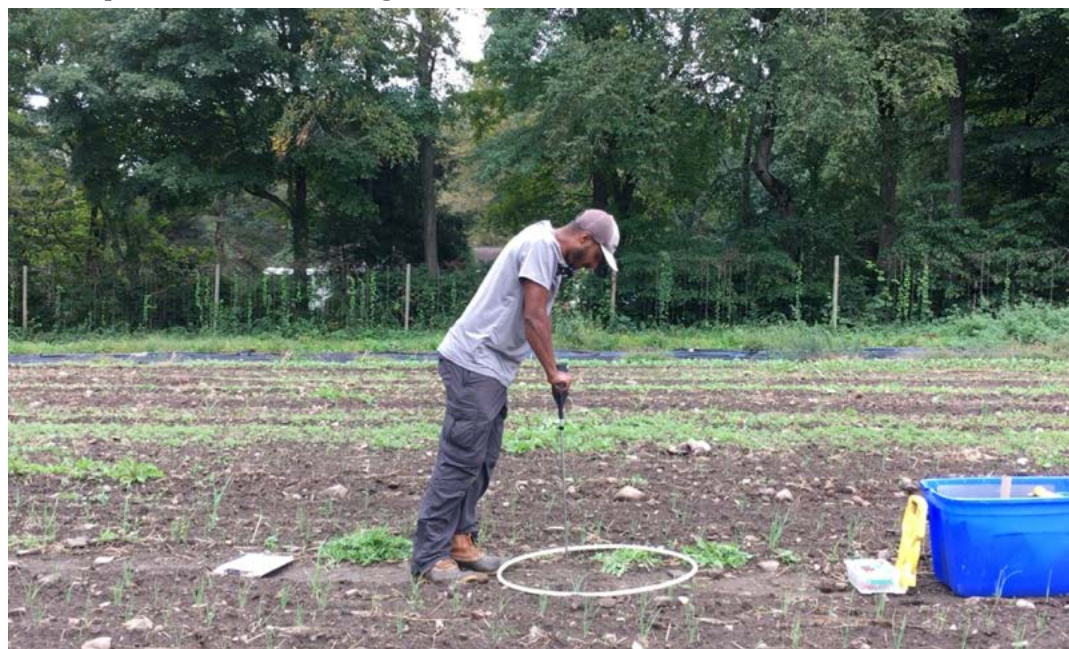
Rubén Parrilla using a soil penetrometer at Assawaga Farm, CT. Photo credit: Monique Bosch
